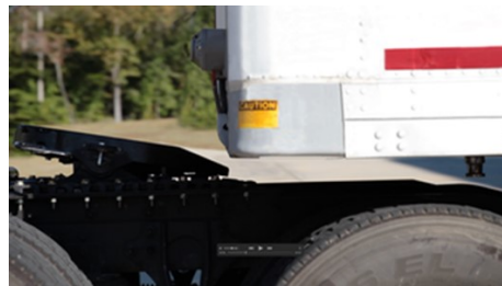
Correct kingpin height before coupling to a trailer
