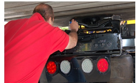
Inspecting the jaws and kingpin connection once coupled to the trailer
